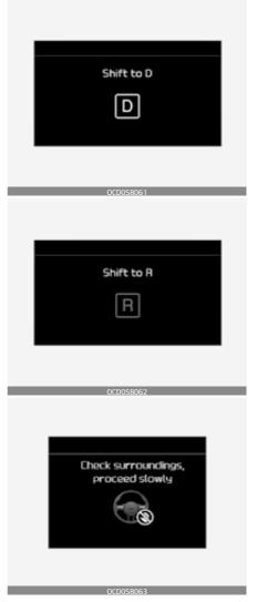
The above message will appear if the shift lever is in D (Drive) or R (Reverse) according to the distance of the front and rear object from the sensor. The steering wheel will be controlled automatically.
