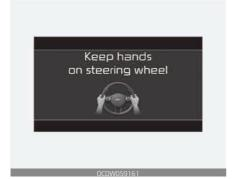
If you keep your hands off the wheel while driving with the LFA system assisting the steering, the hands-off warning will be triggered.
