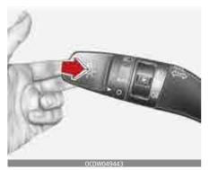
The headlight switch does not need to be on to use this flashing feature.
