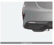
If the rear fog lamp (LED) (1) does not operate, have your vehicle checked by a professional workshop.
