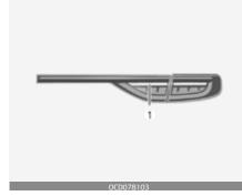
If the rear back up lamp (LED) (1) does not operate, have your vehicle checked by a professional workshop. Kia recommends to visit an authorized Kia dealer/service partner. The LED lamp cannot be replaced as a single unit because it is an integrated unit. The LED lamp has to be replaced with the unit.
