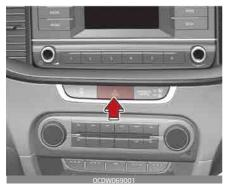
The hazard warning flasher serves as a warning to other drivers to exercise extreme caution when approaching, overtaking, or passing your vehicle. It should be used whenever emergency repairs are being made or when the vehicle is stopped near the edge of a roadway.
