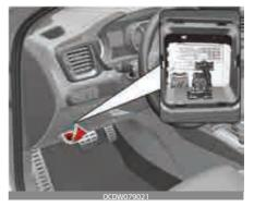
3. Pull the suspected fuse straight out. Use the removal tool provided in the main fuse box in the engine compartment.
