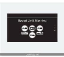
• The ISLW cluster displays not only the no passing and speed limit sign, but also specific speed limits by certain conditions. No reliable speed limit information
