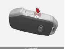
Releasing the tailgate open/ close button (4) on the key stops tailgate movement with the buzzer sound approximately for 5 seconds.
