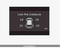
When the tire pressure monitoring system warning indicators are illuminated and warning massage displayed on the cluster LCD display, one or more of your tires is significantly under-inflated. The low tire pressure position telltale light will indicate which tire is significantly under-inflated by illuminating the corresponding position light.
