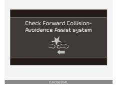
When the FCA is not working properly, the FCA warning light (>>>>) will illuminate and the warning message will appear for a few seconds. After the message disappears, the master warning light (A>>>) will illuminate. In this case, have the vehicle inspected by a professional workshop. Kia recommends to visit an authorized Kia dealer/service partner.
