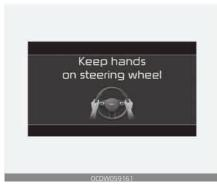
If the driver takes hands off the steering wheel for several seconds while the LKA is activated, the system will warn the driver.
