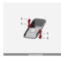
• Pressing or pulling up the power window switch momentarily to the second detent position (6) completely lowers or lifts the window even when the switch is released.
