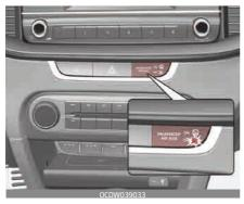
The passenger's front air bag OFF indicator illuminates for about 4 seconds after the ignition switch is turned to the ON position.
