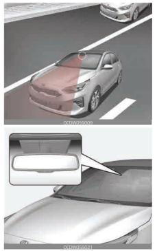
When the system detects the vehicle straying from its lane or road, it alerts the driver with a visual and audible warning, while applying a slight counter-steering torque, trying to prevent the vehicle from moving out of its lane or road.
