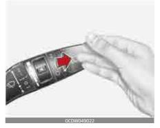
Push the lever away from you to spray rear washer fluid and to run the rear wipers 1 ~ 3 cycles. The spray and wiper operation will continue until you release the lever.
