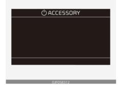
Press the ENGINE START/STOP button when the button is in the OFF position without depressing the clutch pedal.
