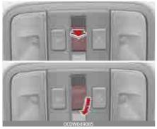
Push the sunroof control lever forward to the first detent position, the sunroof glass will close automatically.
