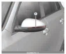
If the side repeater lamp (LED), does not operate, have your vehicle checked by a professional workshop.
