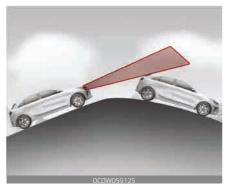
During uphill or downhill driving, the smart cruise control system may not detect a moving vehicle in your lane, and cause your vehicle to accelerate to the set speed. Also, the vehicle speed will rapidly down when the vehicle ahead is recognized suddenly.
