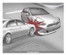
Front air bags may not inflate in side impact collisions, because occupants move to the direction of the collision, and thus in side impacts, frontal air bag deployment would not provide additional occupant protection. However, side and curtain air bags may inflate depending on the intensity, vehicle speed and angles of impact.
