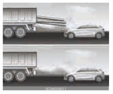
When the vehicle in front has heavy loading extended rearward, or when the vehicle in front has higher ground clearance, it may induce a hazardous situation.
