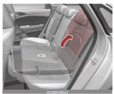
1. To use the rear seat, lift and pull the seatback backward. Pull the seatback firmly until it clicks into place. Make sure the seatback is locked in place. When you return the seatback to its upright position, always be sure it has locked into position by pushing on the top of the seatback. If you can not see the red line at the bottom of folding lever, it means the seatback is locked completely.
