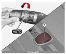
When the light switch is in the AUTO light position, the taillights (bulb type) and headlights will be turned ON or OFF automatically depending on the amount of light outside the vehicle.
