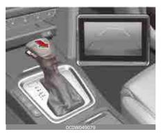
The Rear view monitor will activate when the engine is running and the shift lever is in the R (Reverse) position.
