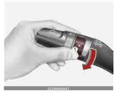
To turn the rear fog lights on, turn the rear fog light switch (1) to the on position when the headlight is turned on.
