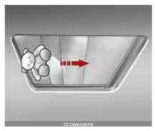
If a object or part of the body is detected while the sunroof glass is closing automatically, it will reverse the direction, and then stop.
