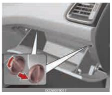
2. With the glove box open, pull the support strap (1).
