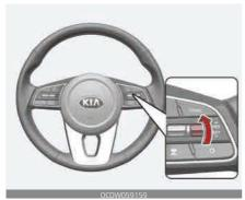
If any method other than the CRUISE button was used to cancel cruising speed and the system is still activated, the most recent set speed will automatically resume when you move the lever up (to RES+).
