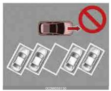
The system is a supplemental for parallel parking or perpendicular parking. Diagonal line parking is not available. Even if the vehicle is able to enter the space, do not operate the Parking Assist. The system will attempt parallel parking or reverse (perpendicular) parking.
