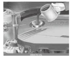
Use a funnel to help prevent oil from being spilled on engine components.
