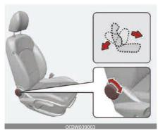
• Turn the control knob forward or rearward to move the seatback to the desired angle.
