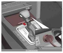
9. Connect between compressor and the vehicle power outlet using the cable and connectors.
