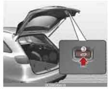
• Press the tailgate open/close button (4) on the key and hold until the tailgate is fully closed.
