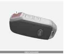
When the vehicle is off, if the door lock button (1) is pressed for 3 seconds or more, the door will be locked and the window will start to move up.
