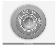
The steering wheel locks to protect against theft. The ignition key can be removed only in the LOCK position.
