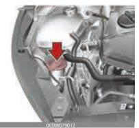
Check the fluid level in the washer fluid reservoir and add fluid if necessary. Plain water may be used if washer fluid is not available.
