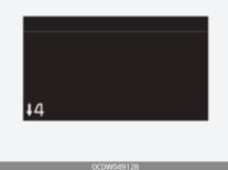
In the Manual shift mode, this indicator informs which gear is desired while driving to save fuel.
