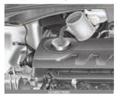
If it is near or at L (Low), add enough oil to bring the level to F (Full). **Do** not overfill.
