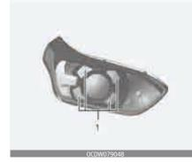
If the position lamp + DRL (LED) (1) does not operate, have your vehicle checked by a professional workshop.
