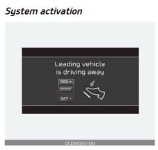
If the driver does not take action for a certain period of time after the vehicle in front departs, the message is displayed on the cluster. The vehicle departs automatically if the accelerator pedal is depressed or [RES +] or [SET -] switch is activated when there is a vehicle in front.
