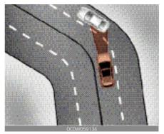
While driving on a curve, the FCA may recognize the vehicle in front in the next lane. Pay great caution, and, if necessary, depress the brake pedal.
