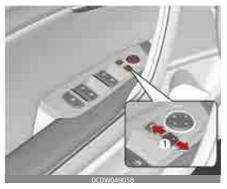
The electric remote control mirror switch allows you to adjust the position of the left and right outside rear view mirrors. To adjust the position of either mirror, the ignition switch should be in the ACC position.
