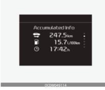
Displays accumulated information starting from mileage/fuel efficiency/time default point.
