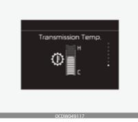
This mode displays the transmission temperature.
