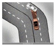
Your vehicle speed can be reduced due to a vehicle in the adjacent lane. Adjust your vehicle speed by depressing the brake pedal according to the road condition ahead and driving condition. Apply the accelerator pedal and select the appropriate set speed. Check to be sure that the road conditions permit safe operation of the smart cruise control.
