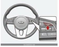
1. Press the CRUISE button on the steering wheel, to turn the system on. The set speed will illuminate.
