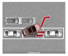
The Parking Assist helps drivers park their vehicle by using sensors to measure parking spaces, control the steering wheel to semiautomatically park the vehicle and provide instruction on the LCD display to help through parking.
