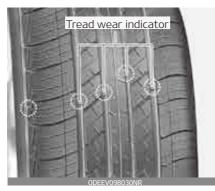
This shows there is less than 1.6 mm (1/16 in.) of tread left on the tire. Replace the tire when this happens.
