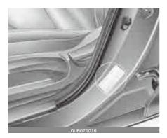
All specifications (sizes and pressures) can be found on a label attached to the vehicle.
