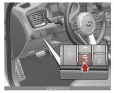
The indicator on the switch will illuminate when the BCW (Blind-Spot Collision Warning) system switch is pressed with the ignition switch ON. If the vehicle speed exceeds 30 km/h (18.6 mph), the system will activate. If you press the switch again, the switch indicator and system will be turned off.
