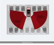
When your vehicle moves backwards from a parking position, the sensor detects approaching vehicles to the left or right side direction and gives information to the driver.
