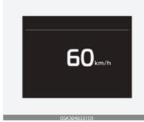
This mode displays the current speed of the vehicle.
