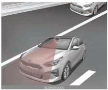
The Lane Following Assist System is designed to center the vehicle in the chosen lane by using a front mounted camera on top of the windshield.
