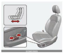
• Push the control switch forward or rearward to move the seat to the desired position. Release the switch once the seat reaches the desired position.
