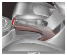
Check the stroke of the parking brake by counting the number of "clicks" heard while fully applying it from the released position. Also, the parking brake alone should securely hold the vehicle on a fairly steep grade. If the stroke is more or less than specified, have the system serviced by a professional workshop. Kia recommends to visit an authorized Kia dealer/service partner.
