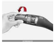
When the light switch is in the parking light position (2nd position), the tail position, license and instrument panel lights will turn ON.
