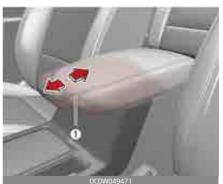
• Grab the front portion of the armrest then press up the lever (1) and pull it forward
