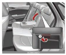
Long objects can be stored by folding the rear center seatback, without having to fold all rear seats. See below steps for folding the rear center seatback.
