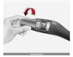
When the light switch is in the headlight position (3rd position), the head, tail, position, license and instrument panel lights are ON.
