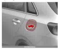
1. To open the fuel filler door, press the 3 o'clock position edge of the fuel filler door.
