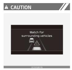
If the vehicle ahead (vehicle speed: less than 30km/h) disappears to the next lane, the warning chime will sound and a message will appear. Adjust your vehicle speed for vehicles or objects that can suddenly appear in front of you by depressing the brake pedal according to the road condition ahead and driving condition.
