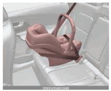
A rearward-facing Child Restraint System provides restraint with the seating surface against the back of the child. The harness system holds the child in place, and in an accident, acts to keep the child positioned in the Child Restraint Systems and reduce the stress to the fragile neck and spinal cord.
