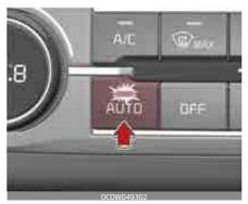
1. Push the AUTO button. The modes, fan speeds, air intake and air-conditioning will be controlled automatically according to the temperature setting.  Front windshield defroster button (Press the button one more time to deselect the front windshield defroster function.
