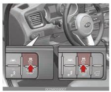
ESC applies the brakes at individual wheels and intervenes in the engine
