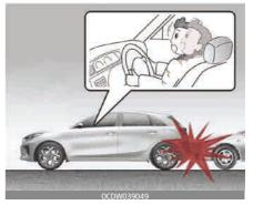
Frontal air bags are not designed to inflate in rear collisions, because occupants are moved backward by the force of the impact. In this case, inflated air bags would not be able to provide any additional benefit.
