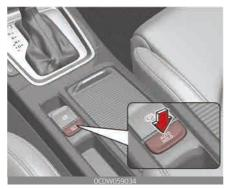
1. With the driver's door, engine hood and trunk closed, fasten the driver's seat belt or depress the brake pedal and then press the Auto Hold button. The white AUTO HOLD indicator will come on and the system will be in the standby position.
