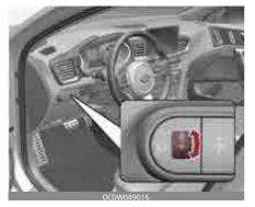
To adjust the headlight beam level according to the number of the passengers and loading weight in the luggage area, turn the beam leveling switch.
