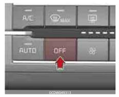
Press the OFF button to turn off the air climate control system. However, you can still operate the air intake buttons as long as the ignition switch is in the ON position.
