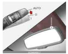
The rain sensor (1) located on the upper end of the windshield glass senses the amount of rainfall and controls the wiping cycle for the proper interval. The more it rains, the faster the wiper operates. When the rain stops, the wiper stops.
