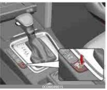
• Press the Parking Assist button (the button indicator will illuminate). • The Parking Assist System will be activated (the button indicator will illuminate).
