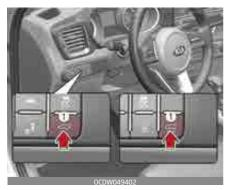
Press the power tailgate close button (3) when the tailgate is opened. The tailgate will close and lock automatically.
