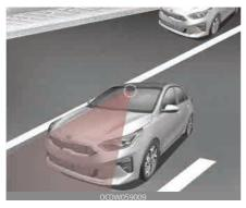
Dirt, snow, or foreign substances on the lens may adversely affect the sensing performance of the sensor.
