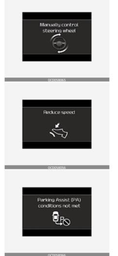
The brake pedal must be depressed by the driver while parking your vehicle. When the Parking Assist is operating, a message may appear regardless of the parking order. The messages will appear according to the circumstances. Follow the instructions provided while parking your vehicle with the Parking Assist.
