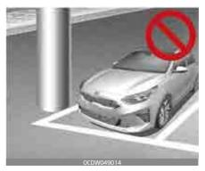
Obstacle such as a pillar may interfere with the system when looking for a parking space. Even though, a parking space is available the system may not detect a parking space.
