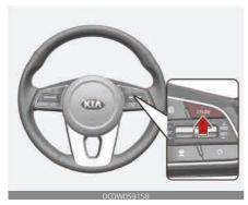
• Press the CRUISE button. (the CRUISE indicator in the instrument cluster will go off).
