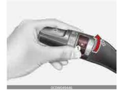
Fog lights are used to provide improved visibility when visibility is poor due to fog, rain or snow, etc. The fog lights will turn on when the fog light switch (1) is turned on after the parklight is turned on.
