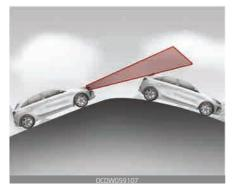
The FCA performance decreases while driving upward or downward on a slope, not recognizing the vehicle in front in the same lane. It may unnecessarily produce the warning message and the warning alarm, or it may not produce the warning message and the warning alarm at all.
