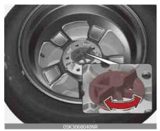
Turn the tire hold-down wing bolt counterclockwise to remove. Store the tire in the reverse order of removal.
