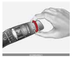
The rear window wiper and washer switch is located at the end of the wiper and washer switch lever. Turn the switch to the desired position to operate the rear wiper and washer.
