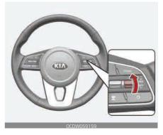
If any method other than the CRUISE button was used to cancel cruising speed and the system is still activated, the cruising speed will automatically resume when you move the lever up (to RES+).
