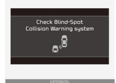
If the system does not work properly, a warning message will appear and the light on the switch will turn off. The system will turn off automatically.
