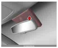
Auto defogging reduces the possibility of fogging up the inside of the windshield by automatically sensing the moisture of inside the windshield and air flow toward the windshield can increase.
