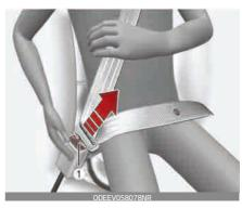
• The seat belt is released by pressing the release button (1) on the locking buckle.
