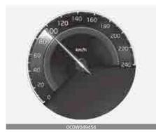
The speedometer indicates the speed of the vehicle and is calibrated in miles per hour (mph) and/or kilometers per hour (km/h).
