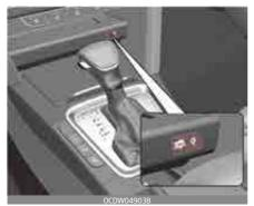
Firmly close all doors, and turn the ignition to ACC or IGN ON. To start wireless charging, place the smart phone equipped with wireless charging function on the wireless charging pad.
