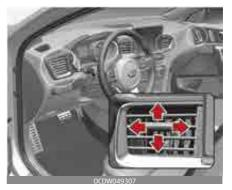
The outlet vents can be opened or closed separately using the thumbwheel. To close the vent, rotate it downward to the maximum position.
