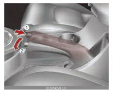
To release the parking brake, first apply the foot brake and pull up the parking brake lever slightly.
