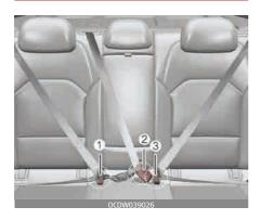
The seat belt should be locked into the buckle on each seat cushion to be properly fastened.
