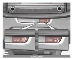
To deactivate the passenger's front air bag, insert the master key into the passenger's front air bag ON/OFF switch and turn it to the OFF position.
